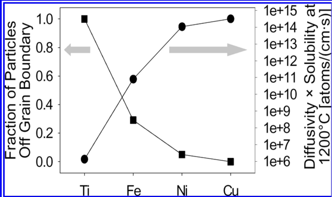
**Cu and Ni** tend to accumulate at a few energetically-favourable regions within the device (e.g., high sigma twins, non-twinning GBs); **Ti and Fe** elements tend to be more dispersed throughout the device. Their low diffusivity also means they are less easily gettered. These facts, combined with their point defect-related deep levels within the bandgap, combine to make these more dangerous for device performance.
