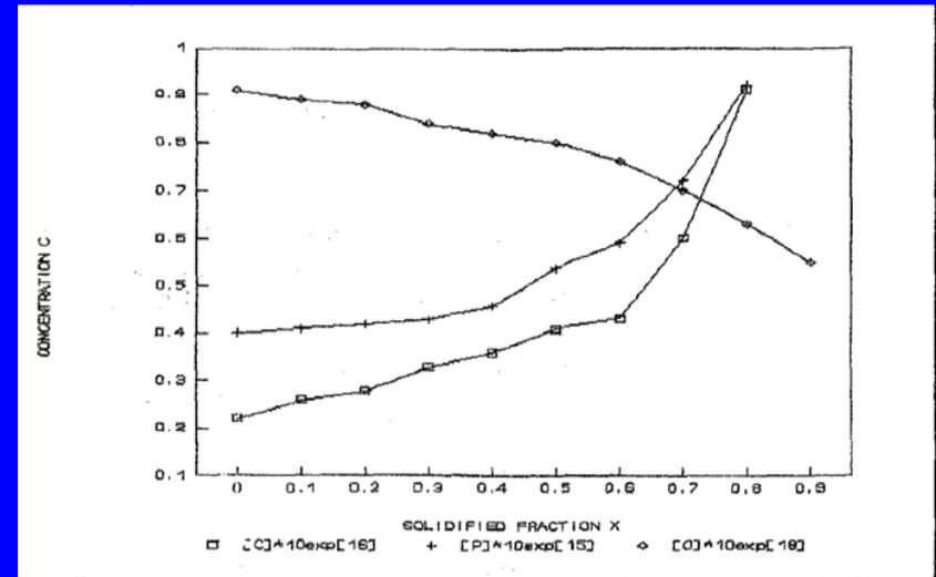
Figure 1. Typical axial distribution of P, O and C content for a 12.5 Kg Cz-Si single crystal ingot
