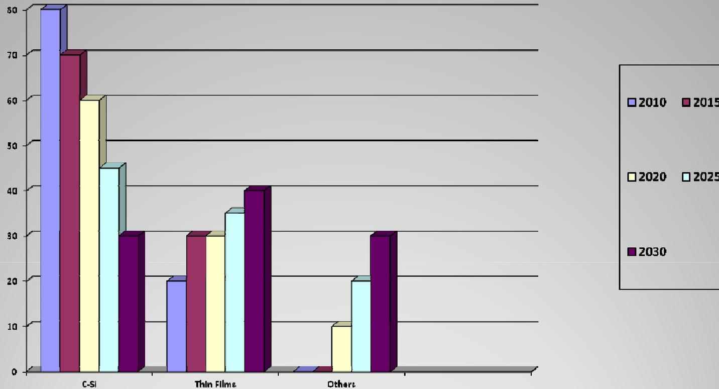
Crystalline silicon (c-Si) modules shared the 85% of the global annual market in 2010 with **module** efficiencies ranging from 12 to >19 %.
