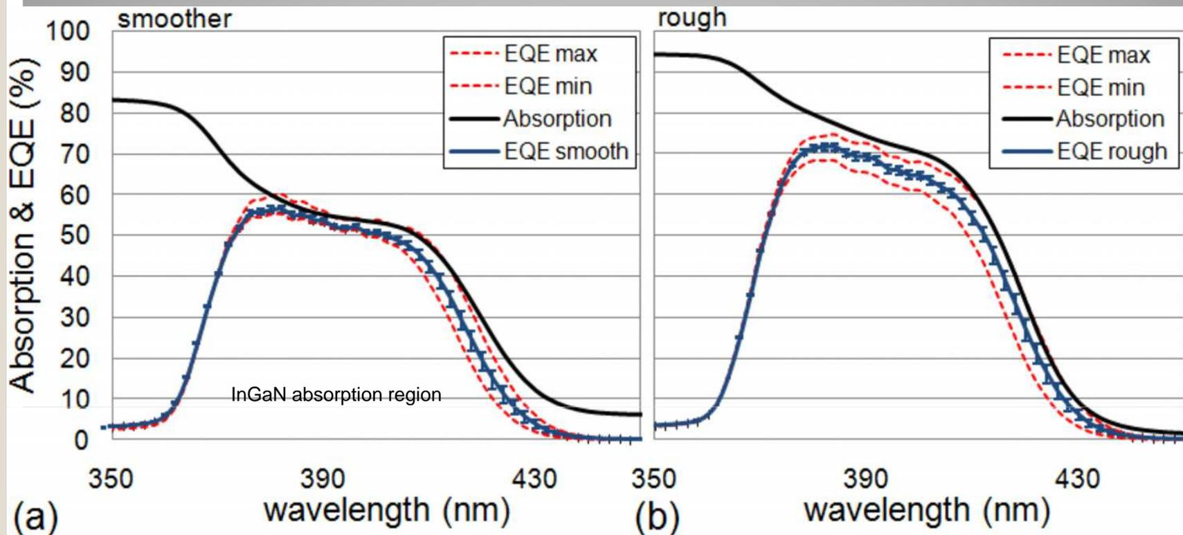
Carrier generation occurs within the InGaN layer with 100% efficiency. Light absorbed in the GaN absorption region ( $\lambda < 365$  nm) EQ=0  $\rightarrow$  100% carrier recombination
